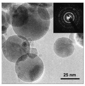
Examples of product nanopowders include simple metal oxides like  $TiO_2$ ,  $Al_2O_3$ ,  $ZrO_2$  as well as complex oxides such as YSZ, CGO, perovskites or spinels. Also, noble metal nanoparticles can be made and deposited onto oxide support particles in the flame. For some compositions, surface-coated or matrix-imbedded nanoparticles can be produced.
